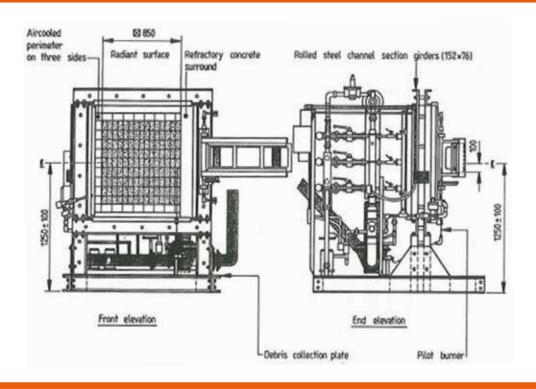
In this method, specimens of the product are subjected to a specific heating process and ignition regime. The test result is a function of the distance and rate of the lateral flame spread, and it is classified according to performance as classes 1 to 4.
